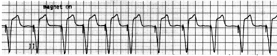
Figure 26–18 Ventricular inhibited pacing (VVI) in the magnet mode, demonstrating the “threshold margin test.” With application of a magnet, this pacemaker (manufactured by Medtronic) generates the first three stimuli at a rate of 100 times per minute. The pulse width of the third stimulus is reduced by 25 percent, but this measurement cannot be made on the routine ECG because of the slow paper speed. The pacing rate after the first three stimuli is identical to that during automatic pacing.
